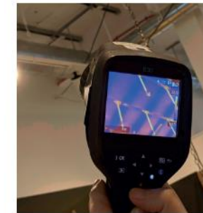
Digital image output from thermal camera identifying the hollow pot slabs of first floor 34 NR.
