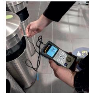
Example of measuring the thickness of a metal object using the ultrasonic thickness gauge.
